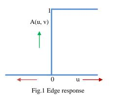
The mathematical representation of amplitude transmission of an opaque straight edge is given by
